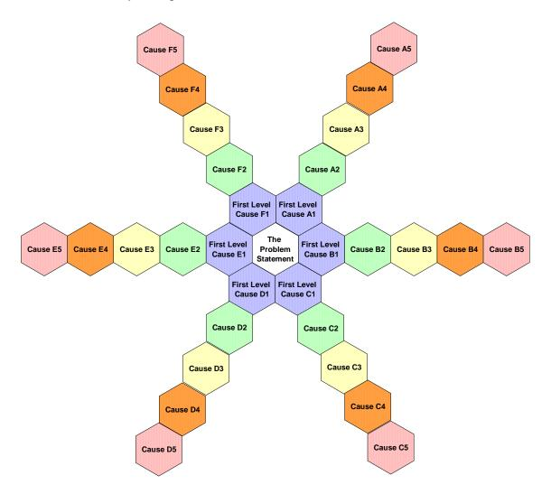
**Step 9**: As the higher level causes are developed, and following the exercise illustrated above, look for causes that appear in more than one place in the diagram. A cause that appears several times is likely to be a root cause candidate.
